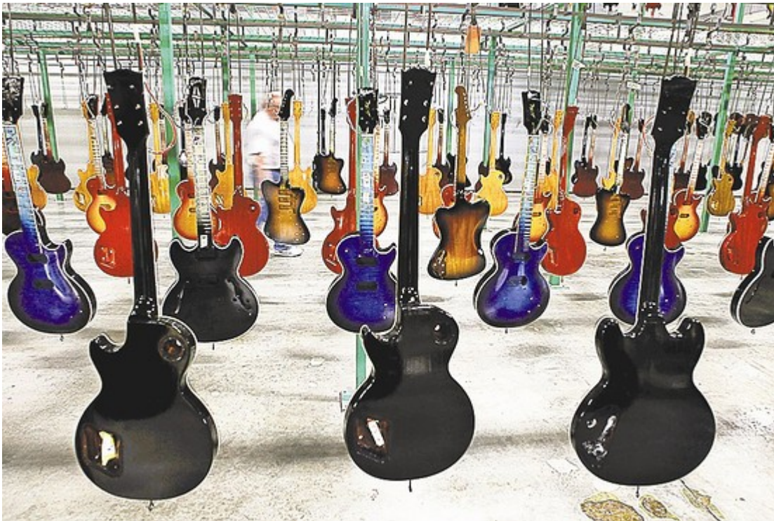
Painted guitars hang to dry after being lacquered at the Gibson Guitar Corp. factory in Nashville, Tenn.
